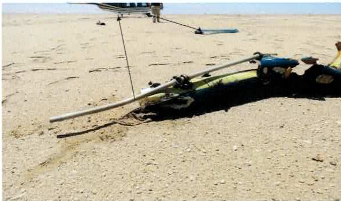
Figure 1. A photo showing the aircraft where it landed and the damage to the tail boom section
