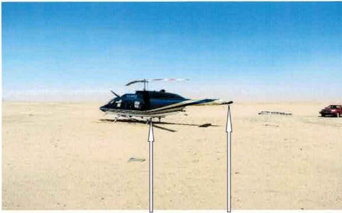
Figure 1. A photo showing the aircraft where it landed and the damage to the tail boom section
