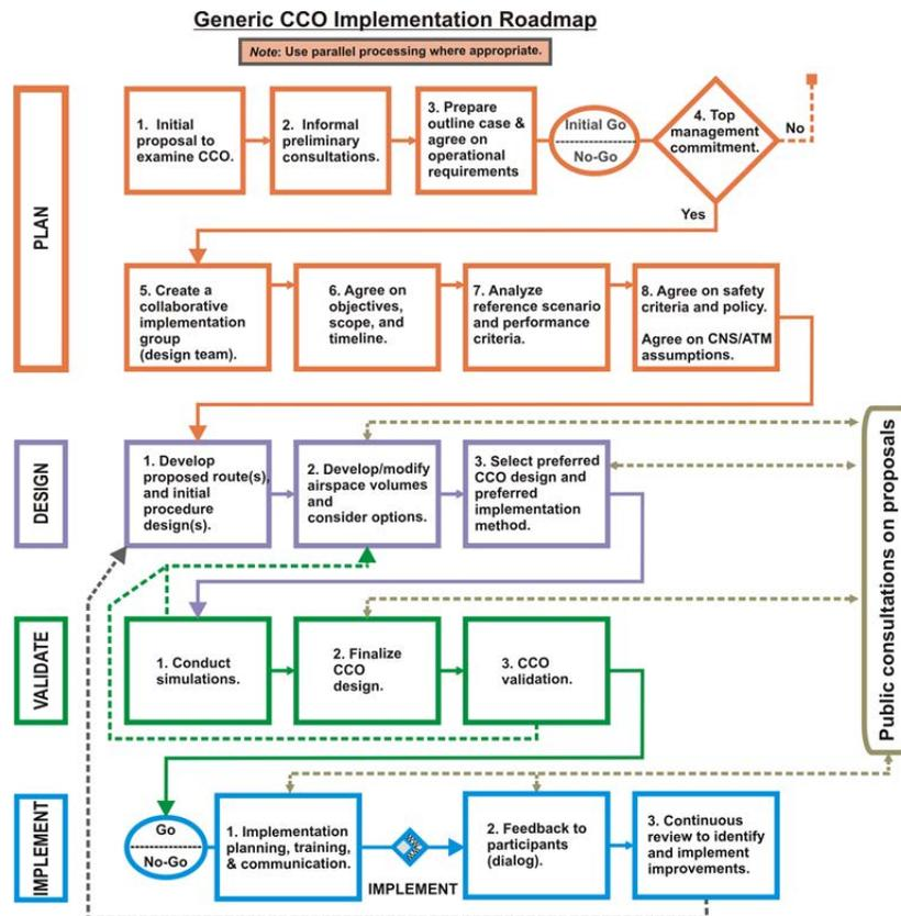
Figure 3.1 CCO Implementation Process Diagram
