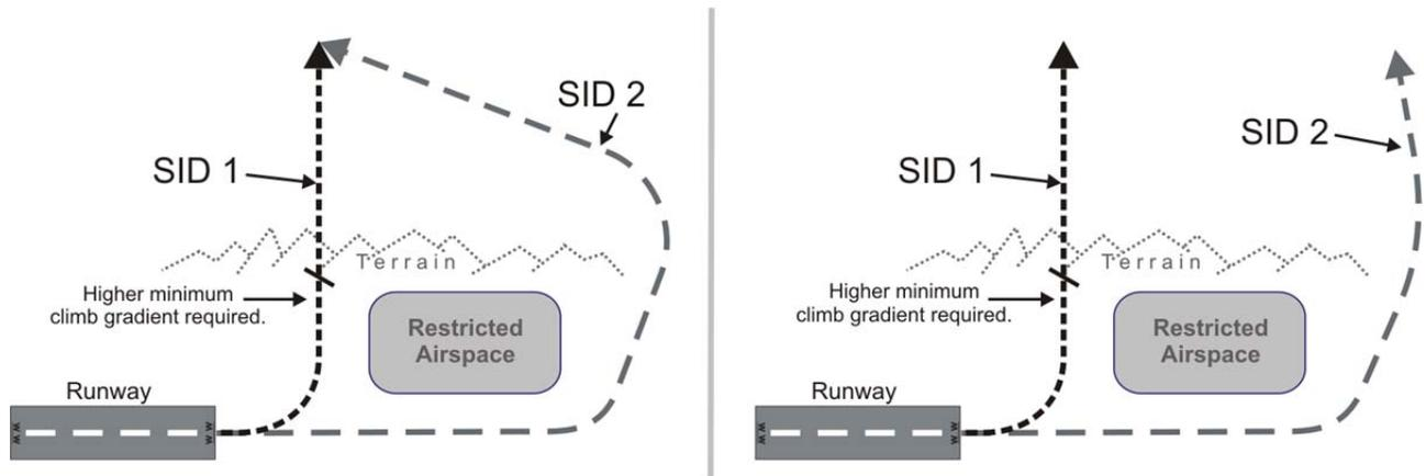
Figure 1.3. Multiple CCO SID Design – Top View
