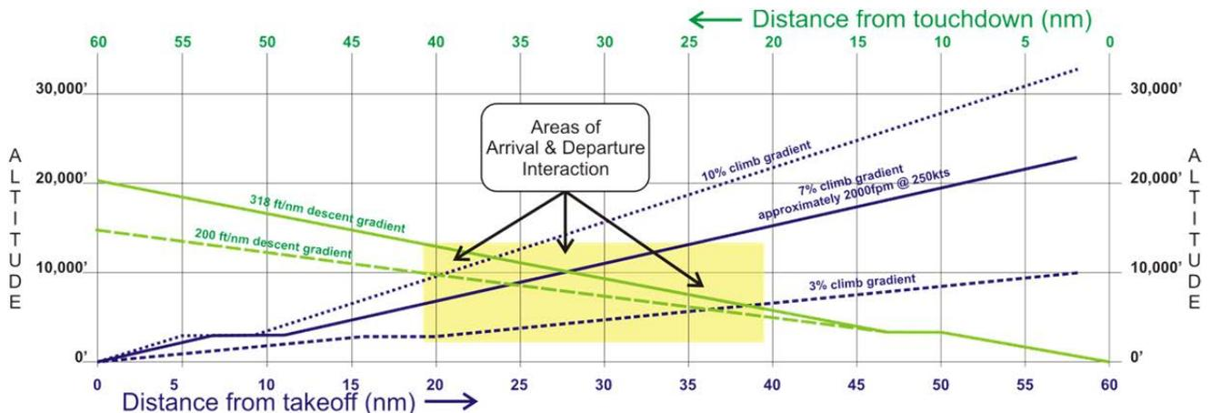
Figure 2.1 Possible Vertical Interaction Between Departing and Arriving Traffic
