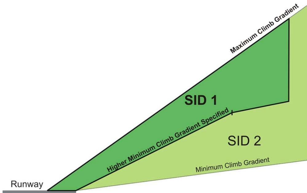
Figure 1.2. Multiple CCO SID Design – Profile View
