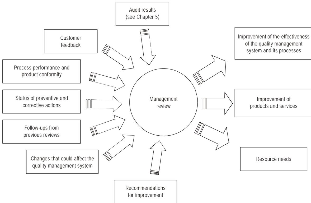
**Figure 3-2. Inputs and outputs of a management review**
